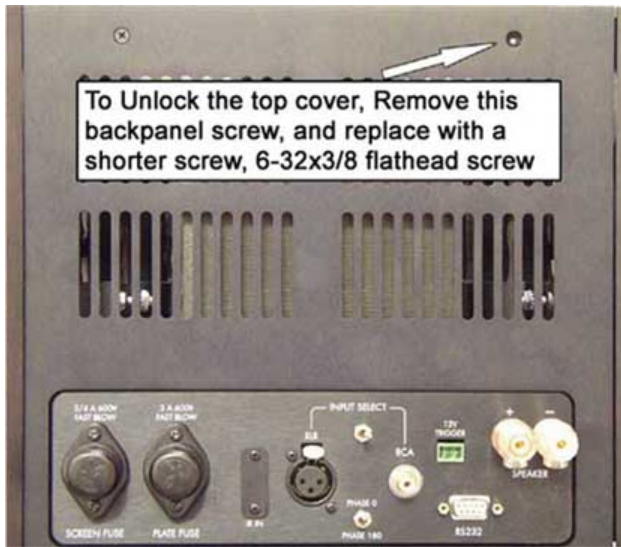
Locations of the Top Cover Screws on the back and side of the Amplifier
